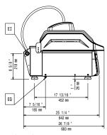
Electrical inlet (power) Electrical Outlet
